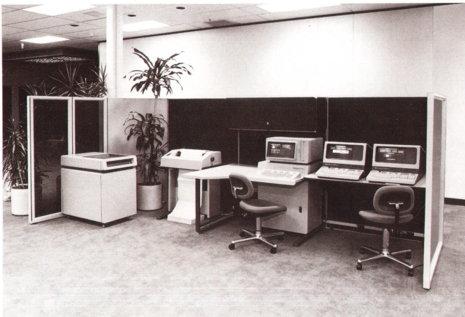
Fig. 1. An HP 300 Computer System including the system unit (center), a printer, two application terminals, and an additional disc drive. Up to 16 terminals, two printers, and 260 megabytes of disc storage can be supported by one system unit.
